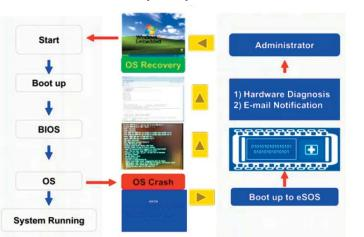
OS. Advantech's Bootsafe Tech firmware causes a Ubuntu-based Linux image to load and boot into recovery mode. The system then runs a variety of diagnostics routines to collect general information into a log file which is then automatically emailed to the administrator.
