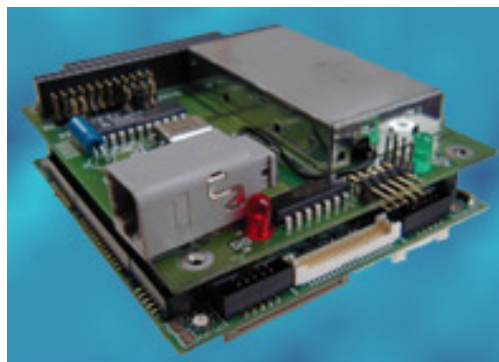
PCM-3291 Mounted on PCM-3346 SBC
